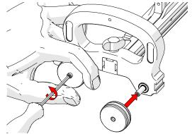
Fig. 30 - Wheel installation
