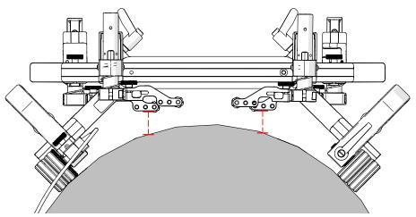
Fig. 104 - Dual pivot frame bar lowered towards scan surface
