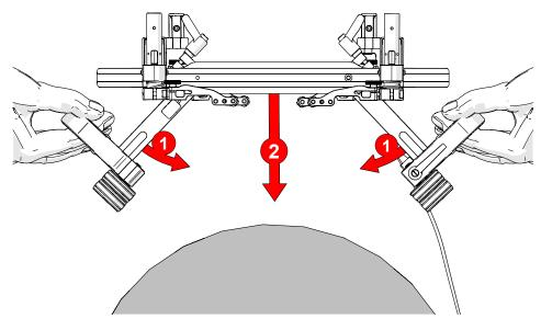
Fig. 97 - Place scanner on scan surface
