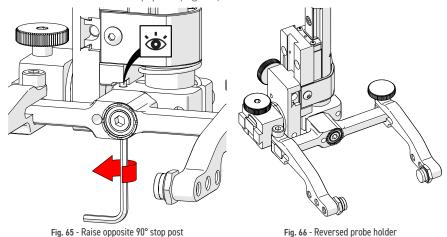
**8.** Raise the stop post on the opposite side until the side of the post contacts the 90° stop point on the probe holder's base (*Fig. 65*).
