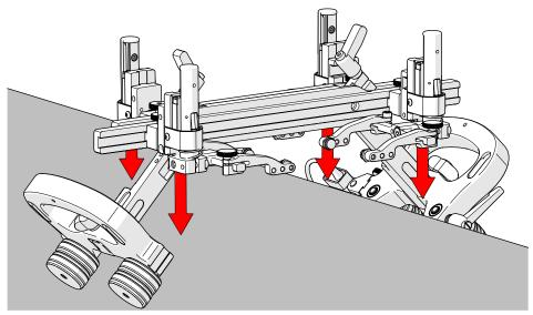
Fig. 100 - Adjust probe holder vertical adjustment
