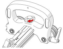
Fig. 25 - Tighten wing knob
