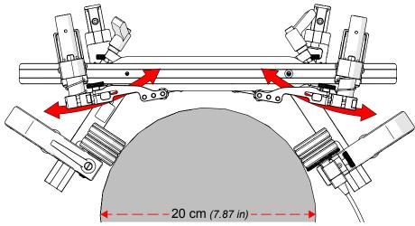
Fig. 102 - Longitudinal probe holder adjustment
