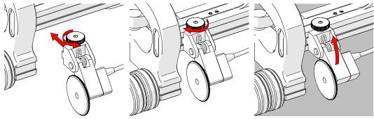
Fig. 39 - Attach to frame bar
