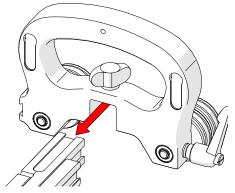
Fig. 24 - Attach to a frame bar
