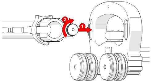
Fig. 69 - Mounting cable management
