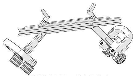
$\label{Fig. 22 - Wheel block with handle, wheels facing outward, handle flush with frame bar} The following indicates the $TIX$ configuration for various scan diameters.$
