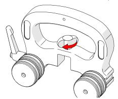
Fig. 23 - Loosen wing knob
