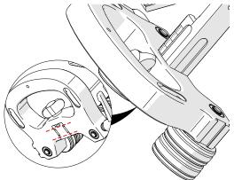
Fig. 29 - Wheel block flush we end of frame bar
