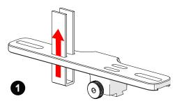
Fig. 81 - Insert velcro straps
