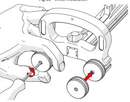
Fig. 31 - Additional wheel installation
