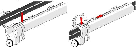
Fig. 70 - Insert cables and hoses
