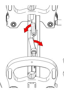
Fig. 94 - Lock dual pivot frame bar levers
