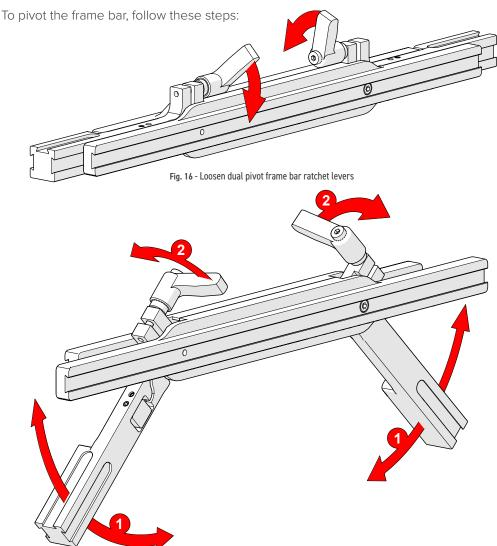
Fig. 17 - Pivot the dual frame bars to required position, lock ratchet levers
