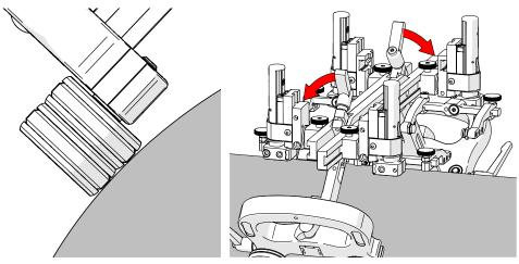
Fig. 98 - Wheels are flat on scan surface
