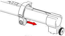
Fig. 75 - Slide clamp onto mount
