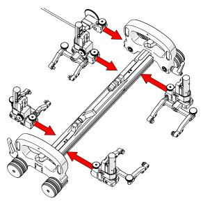
Fig. 90 - Mount probe holders and encoder
