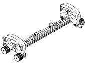
Fig. 3 - Long seam scanner BGA018
