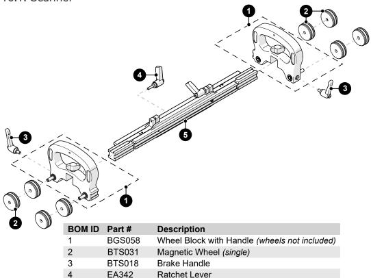
Fig. 105 - STIX scanner parts
