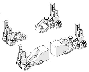
Fig. 88 - Mount probes and wedges to probe holders
