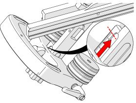
Fig. 28 - Wheel block set to innermost increment
