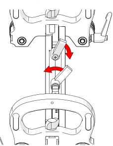
Fig. 89 - Lock dual pivot frame bar levers
