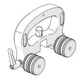
Fig. 19 - Wheel block with handle
