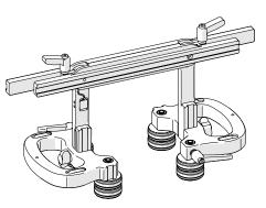
Fig. 26 - Simple wheel block positioning
