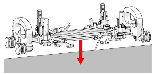
Fig. 92 - Place scanner on scan surface
