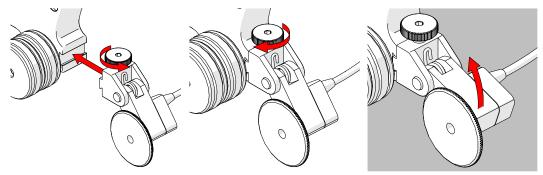
Fig. 36 - Attach to wheel block
