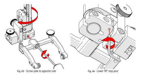
**6.** Mount the yoke to the opposite side of the base using the supplied 3 mm hex driver (Fig. 63).
