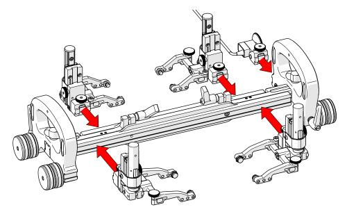
Fig. 96 - Mount probe holders and encoder
