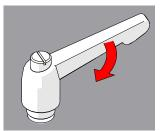
Fig. 35 - Tighten handle
