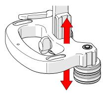
Fig. 27 - Simple wheel block positioning
