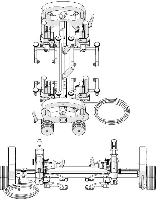
Fig. 85 - Circumferential four probe
