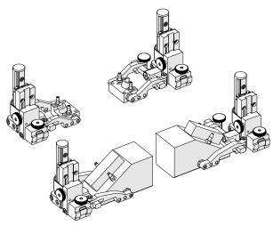
Fig. 93 - Mount probes and wedges to probe holders
