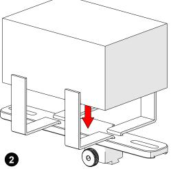
Fig. 82 - Place preamp and wrap velcro
