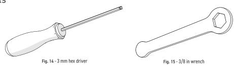
The 3 mm hex driver (Fig. 14) is sufficient for all typical operations and adjustments of the **STIX**.
