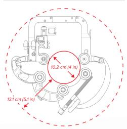
Radial clearance and minimum diameter
