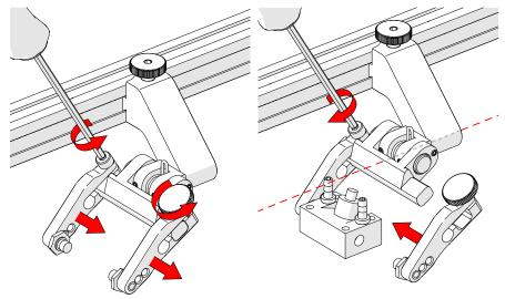
Fig. 36 - Adjust inner probe holder arm
