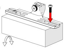
Fig. 44 - Attach preamp with screws
