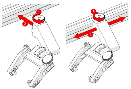
Fig. 34 - Attach to frame bar
