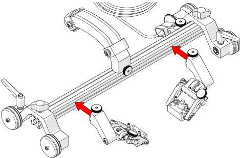
Fig. 49 - Attach spring-loaded probe holders to appropriate configuration
