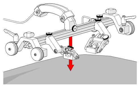
Fig. 51 - Place on scan surface
