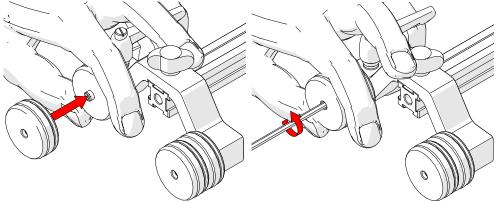
Fig. 40 - Screw on additional magnetic wheel
