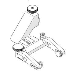
Fig. 4 - Spring-loaded probe holder
