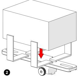
Fig. 46 - Place preamp and wrap velcro
