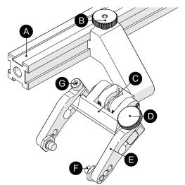
Fig. 33 - Spring-loaded probe holder
