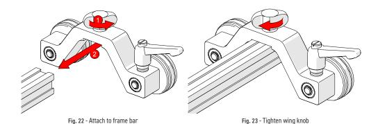
Attach a wheel block by loosening the black wing knob and sliding the wheel block's dovetail nut onto a frame bar (Fig. 22). Tighten the black wing knob (Fig. 23).
