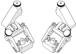
Fig. 48 - Mount wedges to probe holders
