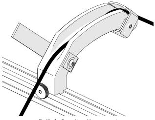
Fig. 18 - Handle provides cable management
